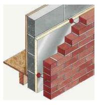
**Durabase galvanized steel modular wall system** – Consisting of a three part outer layer (Brick slip, high density insulation board, structural ply backing panel) and a galvanised steel frame with holes pre-cut to provide access for wiring and plumbing.
